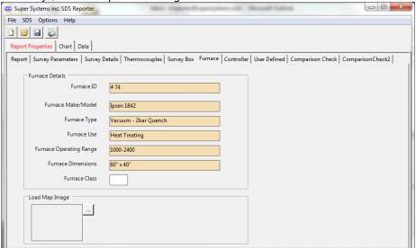
Figure 23 - Report Properties Furnace Tab
