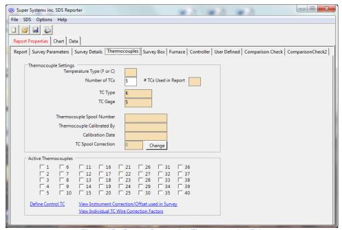
Figure 17 - Report Properties Thermocouples Tab
