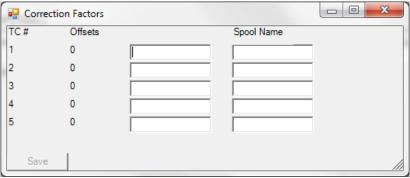
Figure 21 - Viewing and Editing Individual TC Correction Factors
