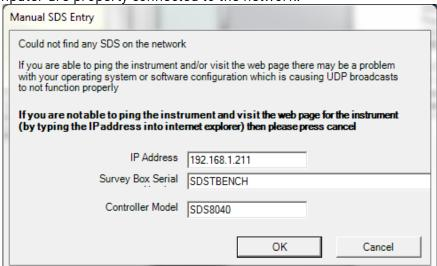
Figure 35 - Manual SDS Entry box
